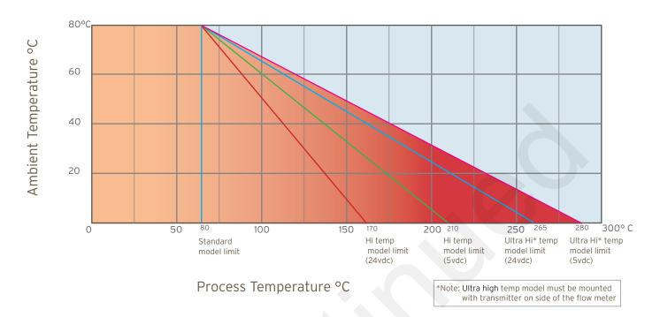
Temperature Limits Model 294 Transmitter Series
