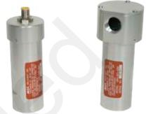
These transmitters are typically mated to a mechanical flow meter, configured, and calibrated at the factory as a matched set. This ensures accuracy and allows quick setup in the field. For field installations where the transmitter has not been setup with a meter at the factory, an optional serial interface kit provides full access to all configuration options and parameters.
