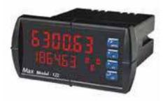
Local process visualization and totalization comes in a standard panel mount display. Input is a frequency transmitter meter and the indicator provides a 4-20mA output for data collection. Displayed flow rate and total are programmable to any engineering units. Easy to program with the on-board software accessed via USB port.
