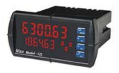
Local process visualization and totalization comes in a standard panel mount display. Input is a frequency transmitter meter and the indicator provides a 4-20mA output for data collection. Displayed flow rate and total are programmable to any engineering units. Easy to program with the on-board software accessed via USB port.
